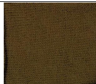
Stocking stitch. Tension 7. 60 stitches x 90 rows (washed)
