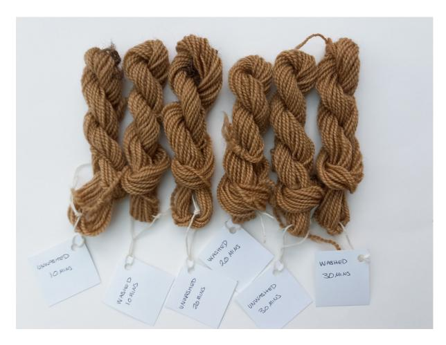
In conclusion: the yarn does bloom with washing and during the natural dyeing process; there is no visible difference in the uptake of dyestuff between washed and unwashed skeins at10, 20 or 30 minutes.
