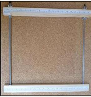
This innovative design enables warp tension to be increased or slackened according need. Easy to use, light weight but robust, the Adjustable Tapestry Frame can be used with G clamps or tapestry frame holders. It can also be broken down into four basic components for ease of carriage and storage (see right). The frame measures approximately 50cm wide with a weaving width of about 35cm. It is 50cm tall. **10 Adjustable Tapestry Frames: £274.50**
